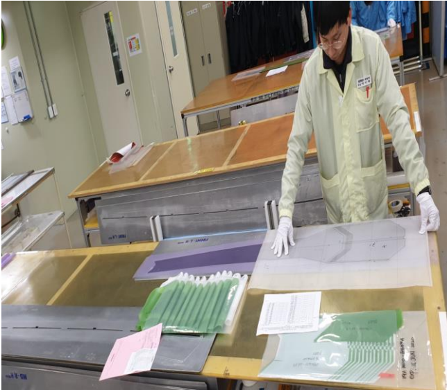
737 MAX SPAR CHANNEL MYLAR INSPECTION
