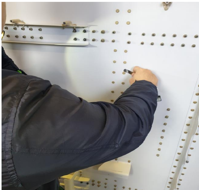
787 AWWB GAP INSPECTION
