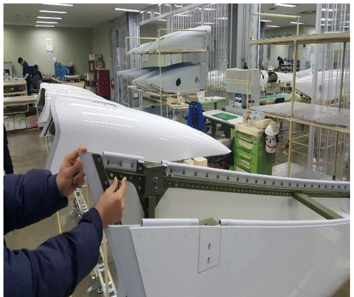
787 FSF PIN PROTRUSION GAUGE INSPECTION
